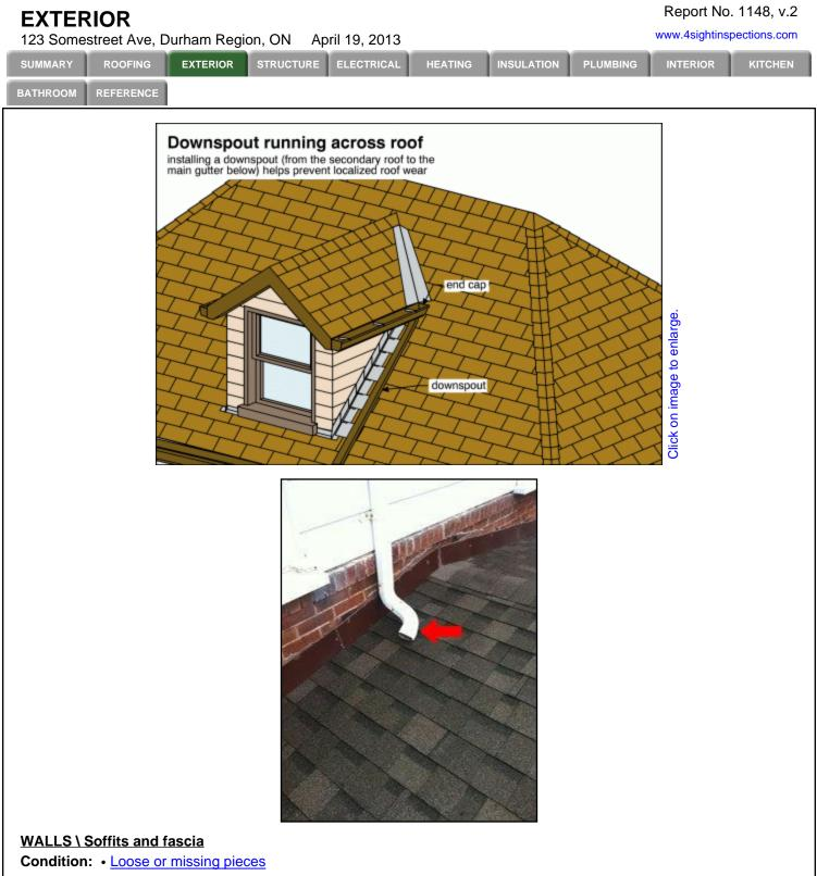
Implication(s): Cosmetic defects | Chance of water damage to contents, finishes and/or structure | Chance of pests entering house Location: Exterior Wall Task: Replace
